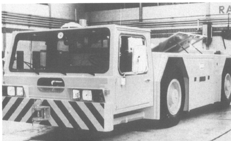
Fig 1 F246 battery-operated aircraft towing tractor
